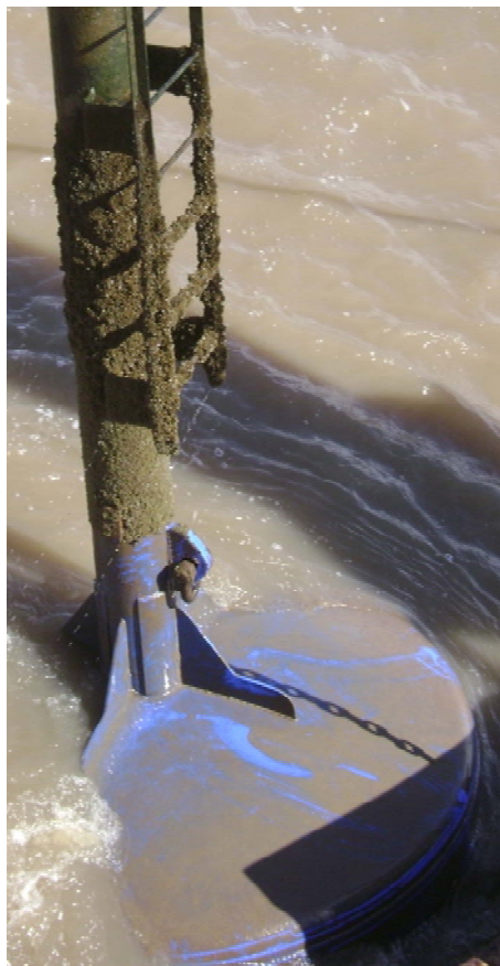
Figure 1 - Spar buoy painted with fluoropolymer paint
